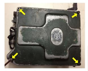
Open the case into two halves and unscrew all the flat head screws with green circles around them (NOT the ones with yellow). There should be thirteen screws in total. Again they are self retaining, so no need to remove them completely. Remove the silica gel packets too. Unscrew the four alan head screws. Do not remove them from the case, they are self retaining.
