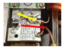
Gently pull all the guts out by levering the orange frequency dial base with a screwdriver and wiggling it all a bit.
