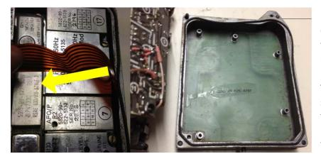
Gently pull orange flexi to remove modules from half of the outer case.
